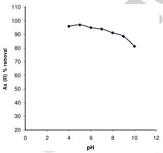
Fig. 3: Effect of pH of solution on As (III) adsorption  $C_{0=}$  1.0 mg l<sup>-1</sup>, adsorbent dose: 25 g l<sup>-1</sup>, shaker speed:130 rpm
