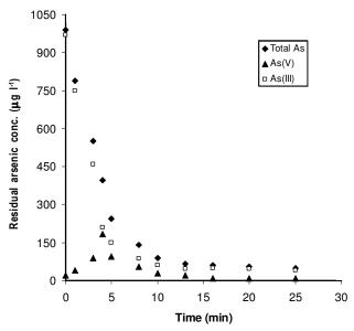
Fig. 4: Speciation study of As (III) on red soil, initial As (III) =1.0 mg  $l^{-1}$ , pH 7.2, adsorbent dose= 25 g  $l^{-1}$ , shaker speed, 130 rpm
