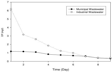
Fig. 7: Influent and effluent OP concentration of municipal and industrial wastewater
