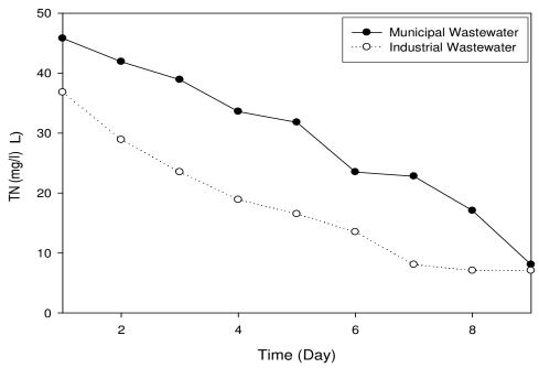
Fig. 3: Influent and effluent TN concentration of municipal and industrial wastewater
