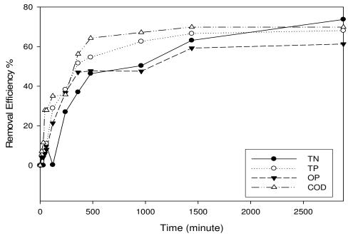
Fig. 10: Changes in removal of COD, TN, TP, OP throughout 48 hr monitoring of municipal wastewater
